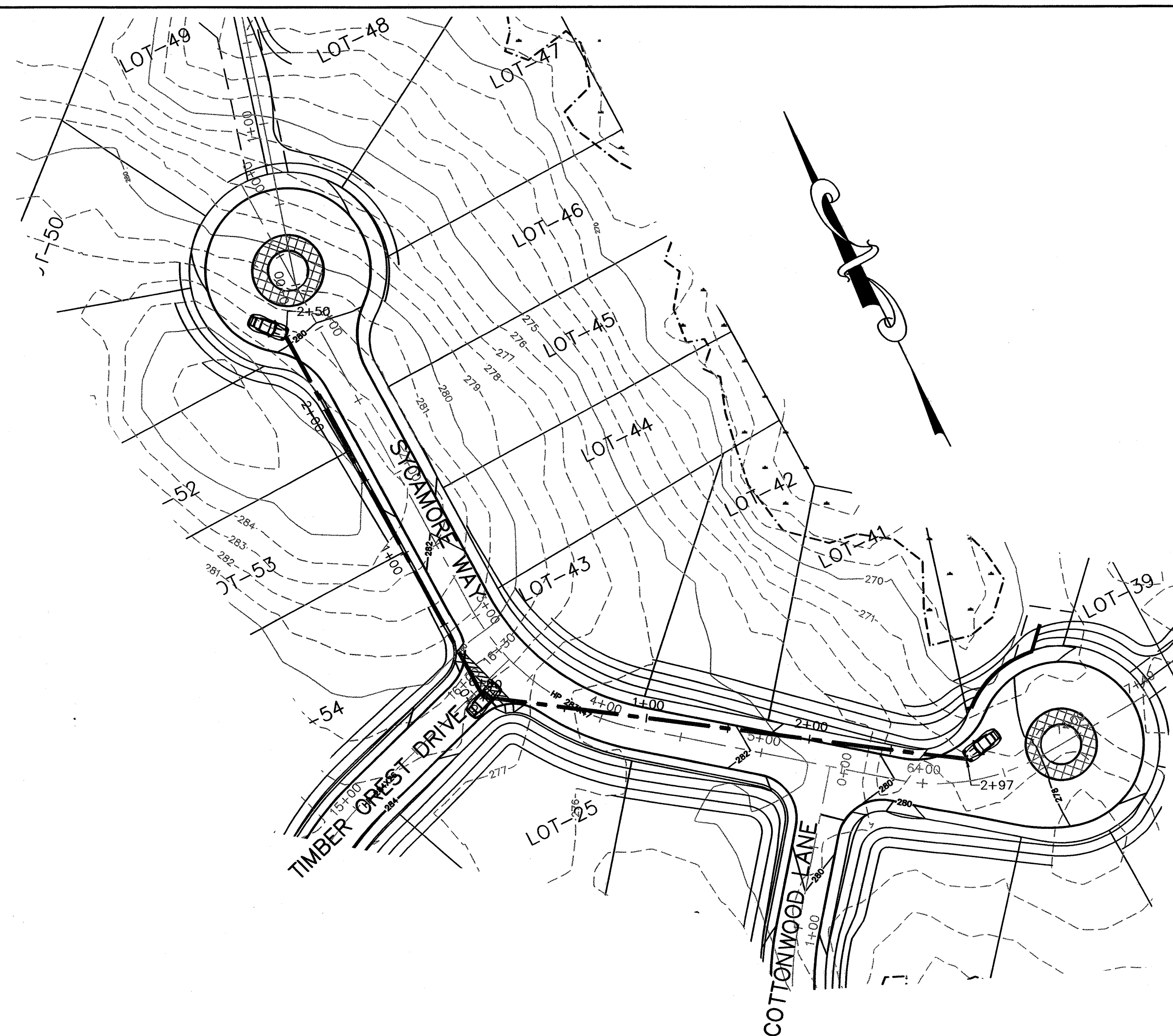
PLAN VIEW OF INTERSECTION SIGHT DISTANCE
